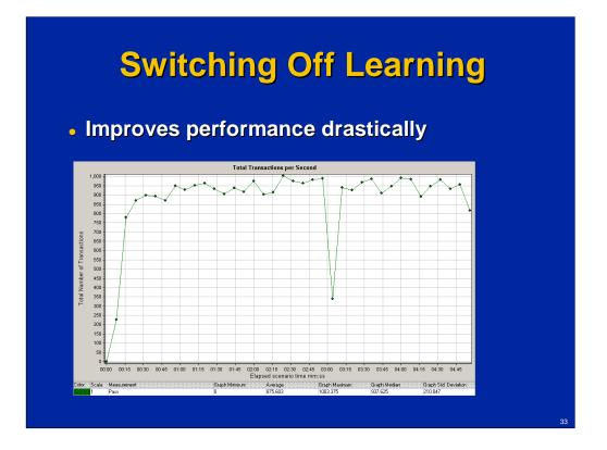
Switching off "learning", the processing of results of all transactions and updating the information used for decision making, improves the performance greatly (up to 876 requests / sec). Although it is definitely not an option for the real deployments: it disables one of the main advantages of the system, self-learning.
