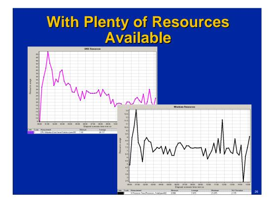
And there were plenty of resources available: with 26.1% CPU utilization on the application server and 7.5% CPU utilization on the database server.
